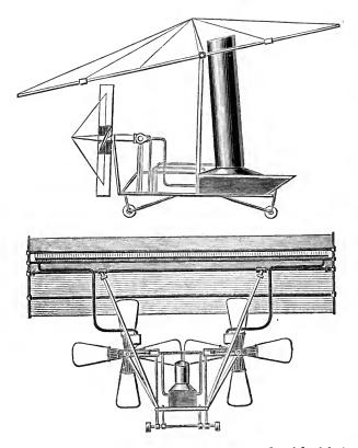
An aëroplane, composed of tubes covered with fabric, is pivotted to the main frame in such a manner that it may be adjusted, up or down, to any required angle.
